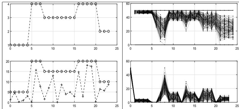
Figure 3.5: Left, top: hourly pumping cost. Left, bottom: upper bounds  $\bar{d}_t$  on hourly demands (o) and sample demand trajectory (+). Right: 100 sample level (top) and control (bottom) trajectories. Pay attention to how close to the tank’s capacity are tank levels in the first five ( $1 \leq t \leq 5$ ) “cheap pumping – low demand” hours and to how intensive is the pumping in the beginning ( $t = 0$ ).
